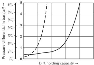
Conventional filter element --(single-layer glass fiber material)
