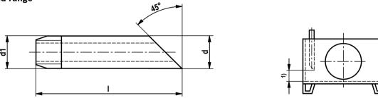
Recommended distance to tank bottom (unless otherwise specified): 60...160 mm [2.4...6.3 inch] From a pipe length of 400 mm [15.75 inch], we strongly recommend fixing the outlet pipe by means of a tank-internal pipe bracket.
