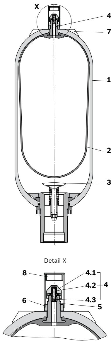
If a certain volume of pressurized gas is charged with a higher fluid pressure, the gas volume will reduce as fluid pressure increases; the gas pressure increases with the fluid pressure.
