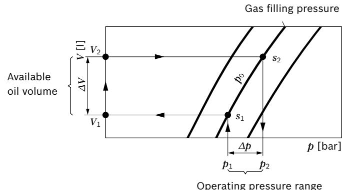
$$\blacktriangleright \text{Isothermal } \Delta V_{\text{real}} = \Delta V_{\text{ideal}} \times K_i$$
